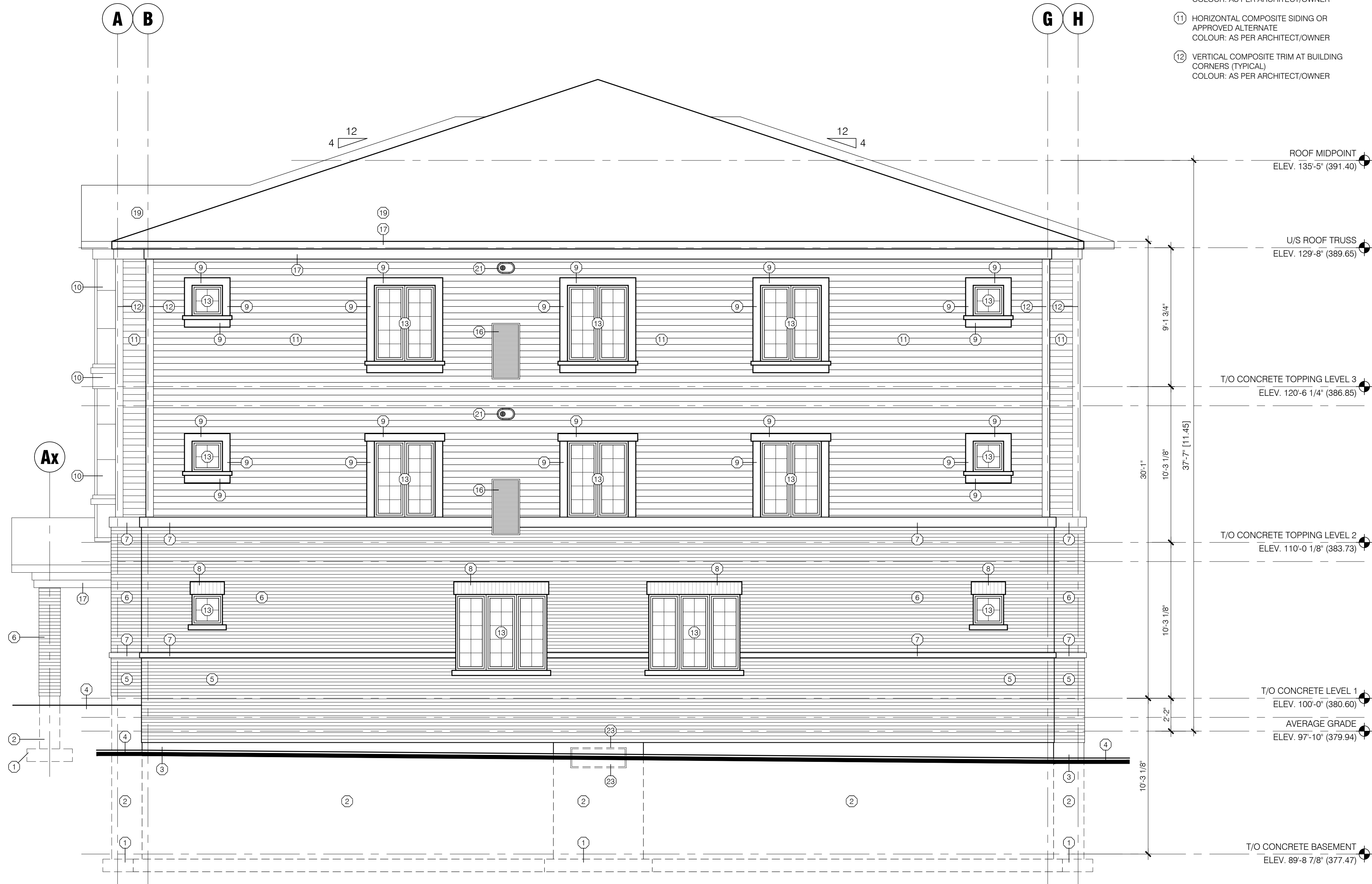
1 WEST ELEVATION - BLOCK 17 A3.2 1/4" = 1'-0"
